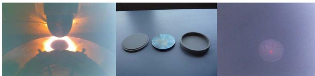
**Figure 1** - Left: Webcam picture of steel disk glowing when heated above 700K. Centre: Steel disk and the ceramic enclosure used to mask its glowing in the visible spectral range. Right: Webcam picture for the ceramic enclosure heated at 750K. The ceramic enclosure is slightly emitting in the visible spectral range, but much lower than the steel disk used previously.
