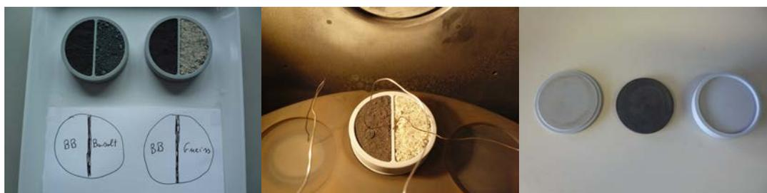
**Figure 2** - Left: Set of ceramic enclosures containing two different samples. Centre: Ceramic enclosure for 2 samples in the emissivity chamber, prepared for measurements (see the temperature sensors on one sample and the
