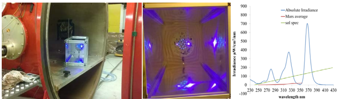
Figure 3. Left: the UV LED system installed into the AWTsII chamber prior to testing at low pressure, centre: view inside the UV chamber during operation, right: a UV-optical irradiance spectrum obtained from within the chamber during operation.
