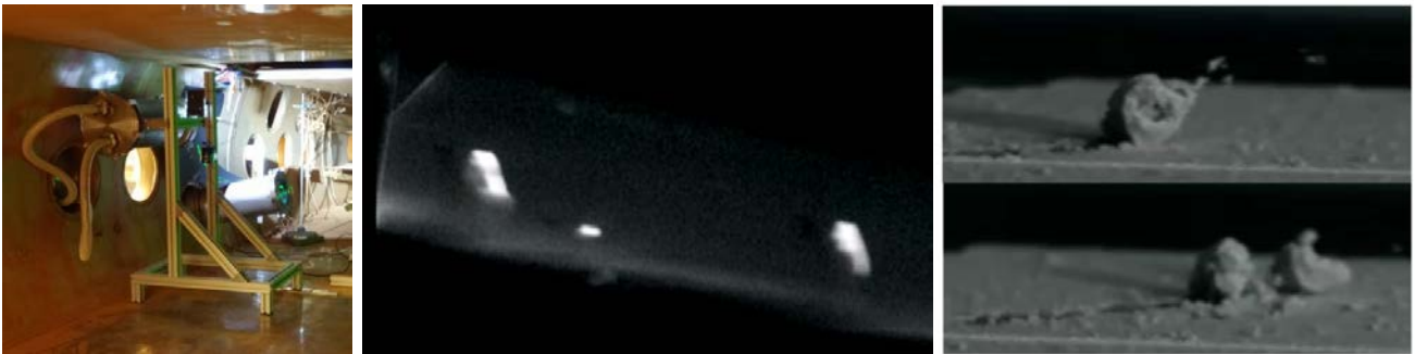
Figure 1 Left: the high speed camera and lighting (laser) system installed within the AWTSII facility (within the pressurized chamber); center: a high speed image of dust and aggregates leaving a 4mm wide nozzle at high velocity into the AWTSII chamber (at 10mbar); Right: high speed images of volcanic ash being removed by wind flow within the AWTSII facility showing rolling sheets of cohered fine ash.
