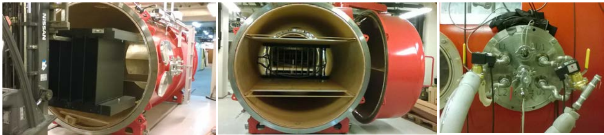
Figure 2 Left: air cooling system being installed into the AWTsII facility; centre: the cooling system (anodized aluminium fins and cooling blocks) having been installed within the wind tunnel; right: the specialized liquid nitrogen inlet/exit flange and valve system.
