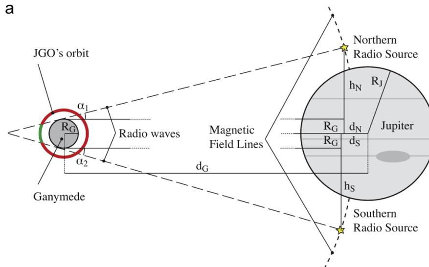
**Figure 4.** Simplified geometry of an orbit of JUICE around Ganymede, with radio source locations. Figure extracted from [Cecconi et al. PSS, 2012](#).
