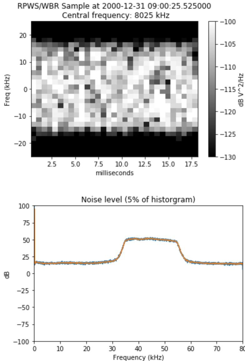
**Figure 6.** Cassini RPWS/WBR examples, extracted from the example jupiter notebook. From top to bottom: waveform, FFT display and noise level spectral shape.
