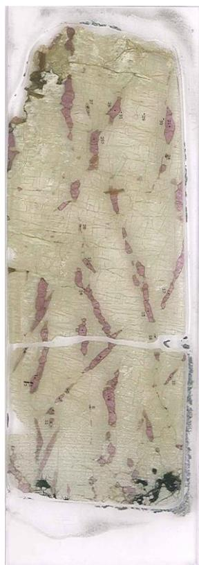
**Fig. 1: Orthopyroxene with garnet exsolution lamellae juxtaposed with granular garnet harzburgite. The Lu-Hf isotope analyses were conducted on the exsolved garnet grains that had been painstakingly separated from the orthopyroxenes.**
