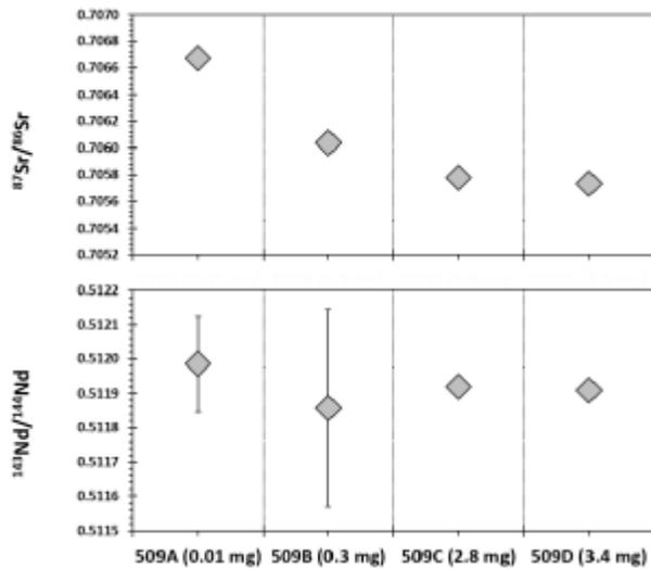
Figure 2. Sr and Nd isotope data obtained on different sized fibrous diamond. These data establish that the Nd blank is almost insignificant but that the current Sr isotope blank requires improvement to allow sub-mg size sample analysis. The Sr isotope data can be used to calculate the isotopic data of the blank and hence allow blank correction of the data from the larger samples, leading to even more precise isotopic data. Typically these correction are less than 1%.
