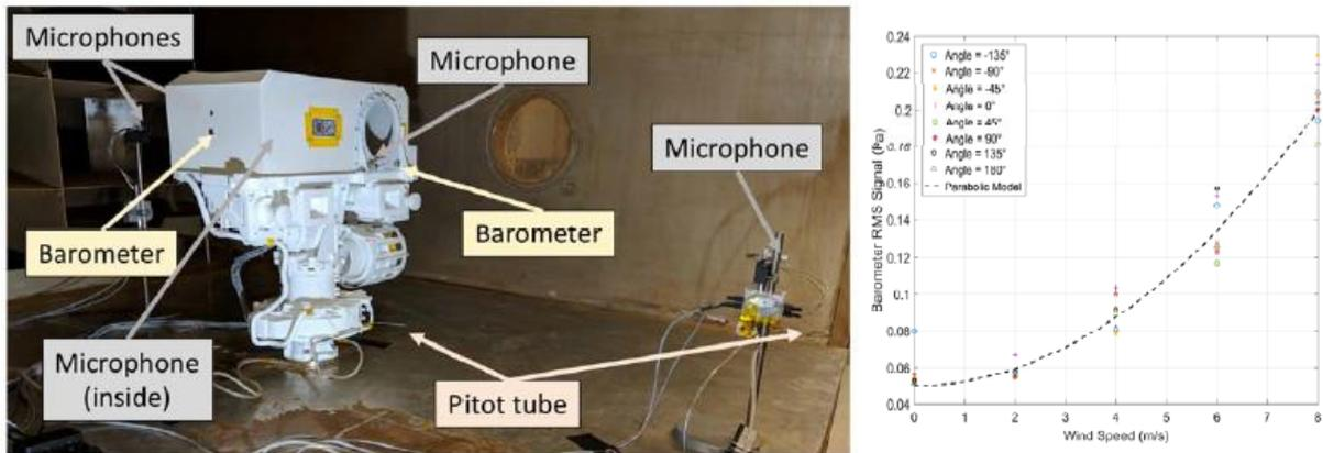
Figure 3- Photograph (left) of the Mars2020 Supercam instrument within the AWTSSII facility being calibrated/tested. Plot (right) shows RMS measurements of the front pressure sensors for varying wind speed in a Martian atmosphere at several SuperCam angles.
