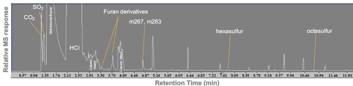
Fig. 1– GCMS run of Lake 2, sample #16. Some relevant peaks identified on the chromatogram. Details of the run conditions in the Dr. Freissinet report.
