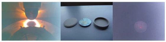
**Figure 1** - Left: Webcam picture of steel disk glowing when heated above 700K. Centre: Steel disk and the ceramic enclosure used to mask its glowing in the visible spectral range. Right: Webcam picture for the ceramic enclosure heated at 750K. The ceramic enclosure is slightly emitting in the visible spectral range, but much lower than the steel disk used previously.
