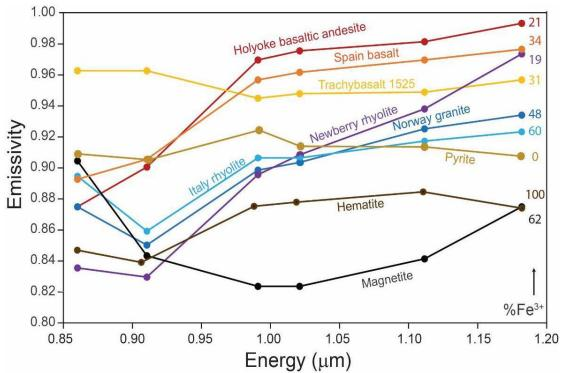
Figure 3 - First set of test measurements for a range of Venus analogues
