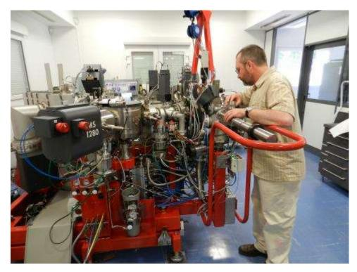
The front end (where solid samples, including polished rock sections are located) of the latest Cameca ims 1280-HR installed at CRPG.
