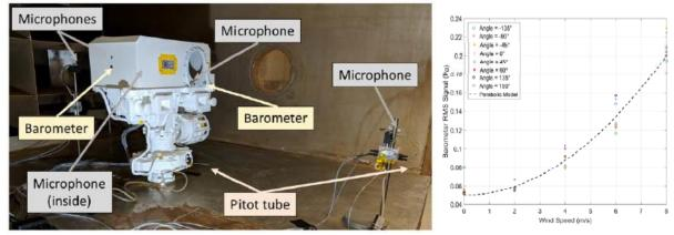
Figure 3- Photograph (left) of the Mars2020 Supercam instrument within the AWTSII facility being calibrated/tested. Plot (right) shows RMS measurements of the front pressure sensors for varying wind speed in a Martian atmosphere at several SuperCam angles.
