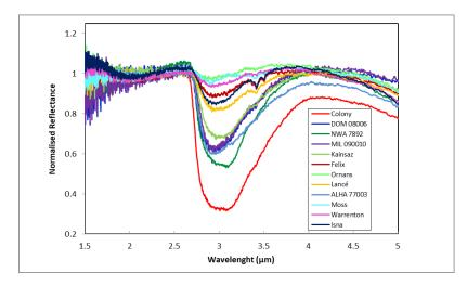
Figure 1 Reflectance spectra showing the 3 µm feature, which is attributed to the presence of –OH/H2O in these meteorites.
