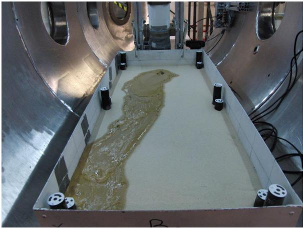
Figure 6: Simulated viscous flow under Mars conditions.
