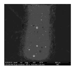
*Figure 5- Experiment A046, produced during the TA visit. The quenched silicate melt is filled with FeSi globules (white) surrounded by FeS. The dark material surrounding the sample is the graphite capsule.*
