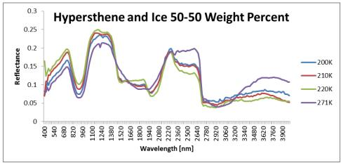
Figure 4- Reflectance spectra taken at different cryogenic temperatures for a 50:50 mixture of hypersthene ice  $(63-125 \mu m)$  and dust.
